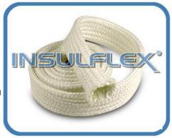
Product Overview: Thermosleeve B is a bulk economy grade fiberglass sleeve that offers maximum thermal efficiency for minimum cost. It is ideal for use as insulation or heat protection of hoses and cables. Thermosleeve B is often used underneath Pyrojacket or Pyreflect sleeve as an effective way of increasing insulation values for minimum cost.
