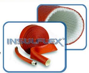
Temperature Capabilities: Rated for 500°F (260°C) to -65°F (-54°C) continuous exposure, up to 2000°F (1093°C) for 15-20 minutes and up to 3000°F (1650°C) for 15-30 seconds.
